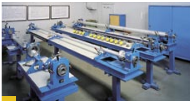
Inspection/measuring equipment for ARIANE 4, PAL-BOOSTER piping
