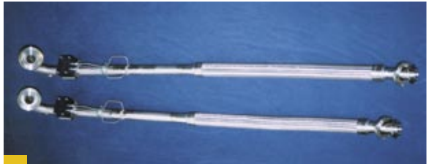
ARIANE 5 EPS feedlines 40 × 2.0 mm/3.18 × 0.51 mm, material grade 1.4546.9
