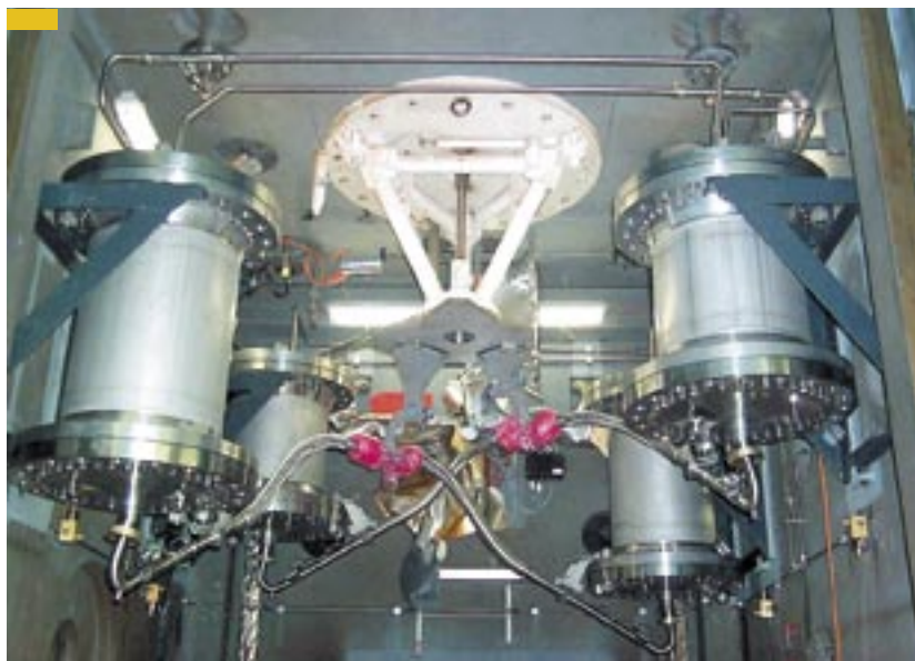
Piping component with pyro valve and burst disk for the residual gas emission in the fuel system of ARIANE 5, EPS-upper stage, in grades 1.4544.9, 1.4546.9, Z4CMN21-06-09, dimension 12 x 2.0 mm
