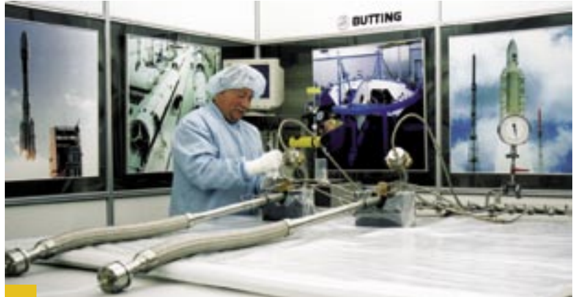
Works in the cleanroom; ARIANE 5 EPS feedlines
