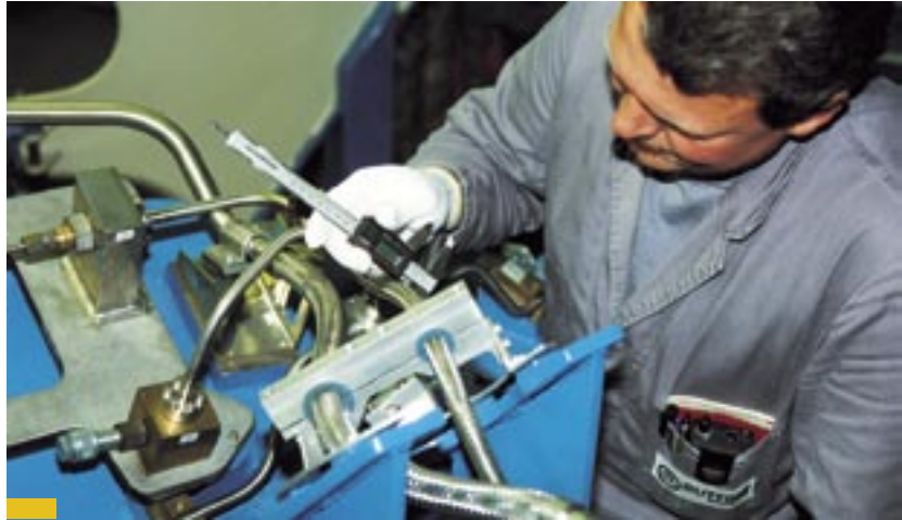
Dimensional control of the ARIANE 5 EPS piping – upper stage
