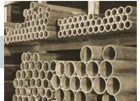
1890 Transition from handcraft to industrial operation (mass production of soldered copper pipes)
