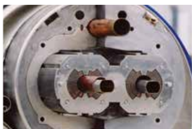
The superconductive magnet is coated by LHC half shells, encasing both beam screen pipes
